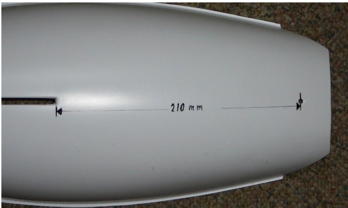
Figure 2: ballast position
