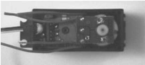
Figure 6. Replace the plastic holder on the circuit board and resolder the center lead of the feedback pot to the pc board. Slide this assembly back into the case routing the wire pairs around the edge of pc board S202-1.
