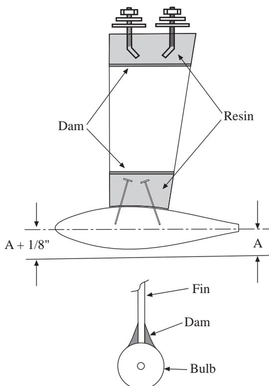
Using filler material (auto body surfacing putty), make a dam around base of blade and top of bulb. Pour approximately 1/2 oz. of epoxy or resin into top of keel blade to cover top of nails. Let epoxy or resin cure.
