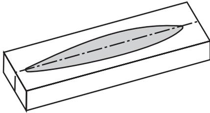
(this will vary with bulb size) balsa wood together. A layer of thin cardboard lightly glued between the blocks makes splitting them apart much easier. The glue joint will be broken apart later.
