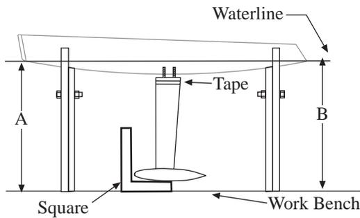
Place masking tape around upper portion of keel fin approximately 1/2" from top. Apply thin layer of slow cure epoxy with a filler (micro-balloons) additive to top outside surface of keel fin. CAUTION: Be sure the epoxy is not close enough to bolts to be forced up into bolt holes when mounting keel.
