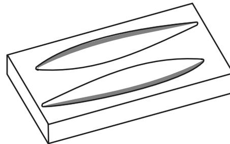
Fill recesses with lead shot (the smaller, the better) and tamp lightly. Thin a quantity of resin (casting resin is best) with acetone. Be sure to catalyze. Pour the resin into the lead shot in both halves.
