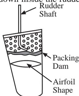
slightly below the rudder shaft. Align the shaft in the rudder so that it is at right angles to the water line of the hull, vertically straight with the rudder sides, also with about 60 % of the rudder area aft of the shaft. When it's in alignment tack glue it with Zap. Now you can fill the inside of the rudder with a filler of micro-balloons and resin or epoxy.
