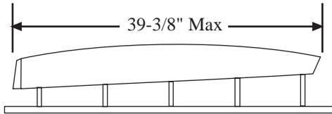
When the hull is planked, nose piece or bumper installed, hull sanded and **BEFORE** you remove the frames, place the hull on a flat surface. Measure the hull for over-all length. The maximum L.O.A. for a One Meter yacht is 39 3/8". Minimum is 39". This is measured parallel to the waterline.
