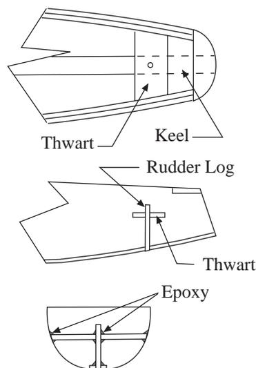
Locate the position of the rudder shaft. Drill a 3/16" hole through the keel and bottom of hull. This hole must be drilled at right angles to the waterline. Insert the correct length of 5/32" I.D. brass tubing through the hole, through the thwart extending above the waterline. Be sure
