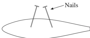
Slip keel blade down over nails. Some sanding will be required to fit the bottom of blade to top of lead bulb. the forward point of bulb should be elevated approximately 1/8" above aft end of bulb.
