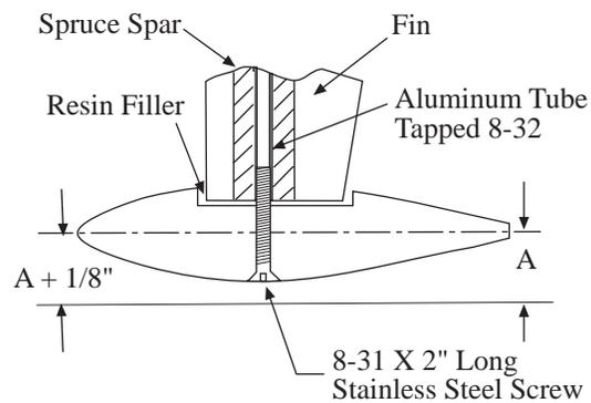
Fill the cavity around the fin with a filler of resin and micro-balloons. Allow to cure for 24 hrs.
