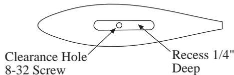
You can make the 1/4" deep recess in the bulb with a moto-tool or rotary bit in a drill motor.
