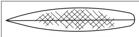
Place 1 oz. fiberglass cloth over dry hull, with fibers running approximately 45° to keel. Smooth out fiberglass cloth with palm of your hand over entire hull (except transom).
