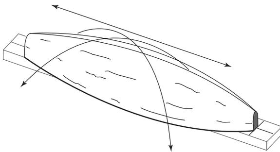
Gently apply resin or epoxy to the hull, starting in center of keel and work toward bow and stern. Apply resin or epoxy to the remainder of the hull using a downward motion and let cure.
